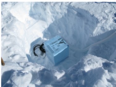
Sensors were insulated from the cold
