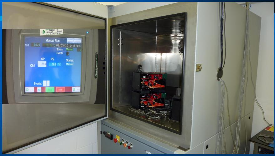
Each and Every one of our instruments is passed through the Environmental Chamber for 7 days to pass the production test. 70 pages report of the digitizers' performance is generated and used to qualify if instrument is ready to go on the shelf/delivery. Rated from -30 to +75C.
