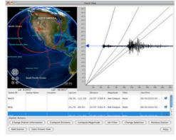
**Event View-** All of the analysis for an earthquake comes together in the event view. Multiple traces can be loaded, either from the stream view or from a sac file. All of the individual distance calculations are displayed in both table and map form in addition to the individual magnitude calculations. In this view, a user can make the final determination of the location and size of the earthquake.
