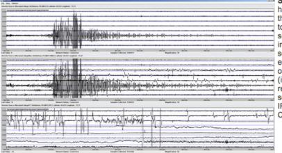
Stream View- The helicorder screen now has the flexibility to display up to three streams of data simultaneously. These can include a local educational seismometer, a remote educational seismometer over the jAmaseis network (in true real-time), or research-quality seismometers stored at the IRIS Data Management Center (in near real-time).
