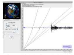
Computing Distance- For each stream, an event can be extracted allowing the user to pick arrivals by double-clicking on the seismogram. A travel time curve is available to align the picks, and as the seismogram is slid along the travel time curve, the numeric values update and a circle with the appropriate radius is shown on the globe.
