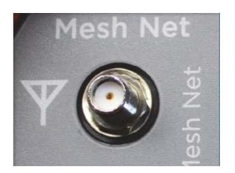
Mesh devices are paired wirelessly with a specific Q8 and data can "hop" via other network nodes in range and give a range of approximately 100m using a 2.4GHz frequency
